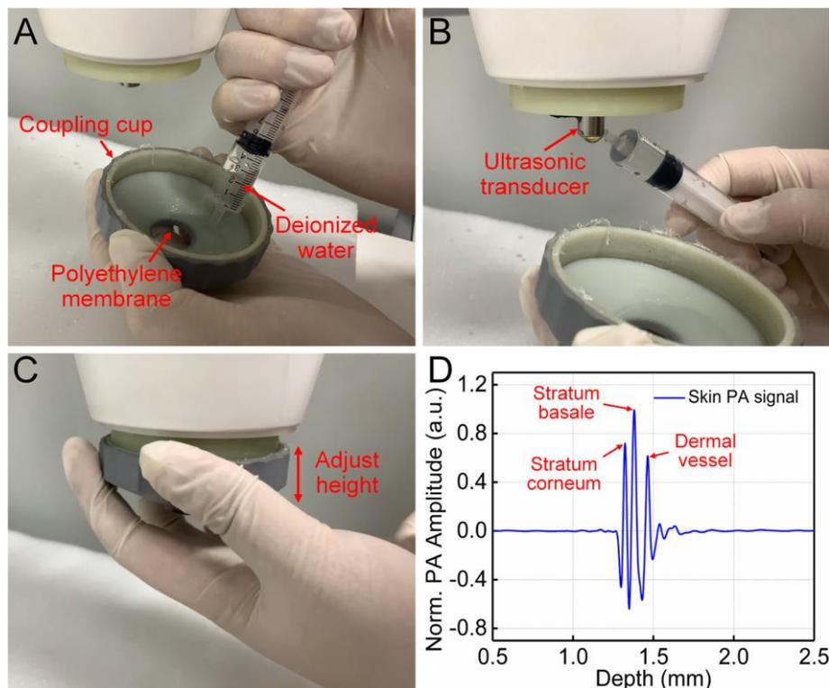
**Figure 3. System alignment and acquisition of skin signals.**
